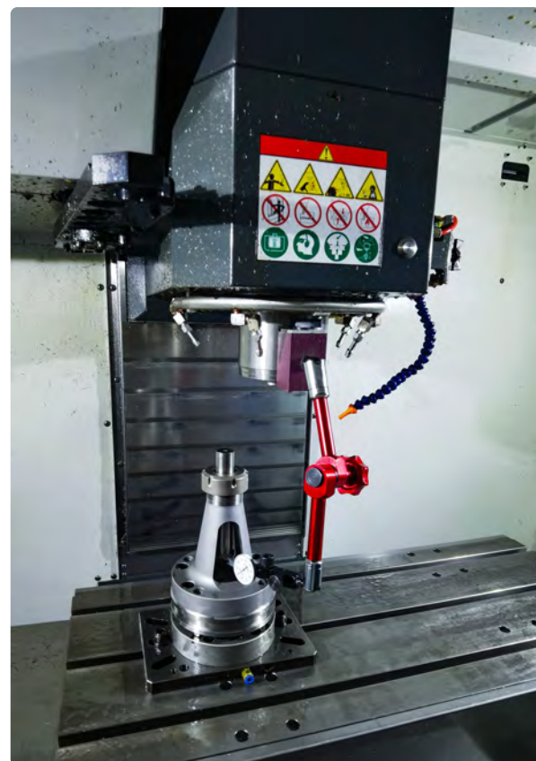
托盘在卡盘上快速装夹定位 Quick clamping and positioning of pallet on chuck
