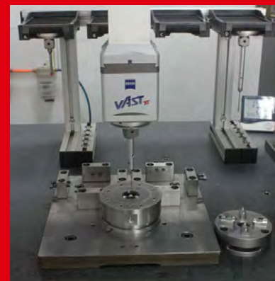
ZEISS三坐标测量仪检测 3A-110004零点卡盘 ZEISS coordinate measuring machine detects Zero Point Chuck 3A-110004
